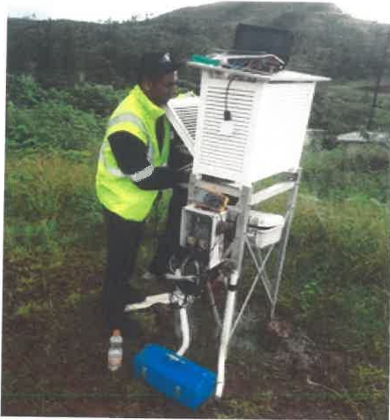
Figure 2: Mr. Ashnil Kumar, AWS Technician with the Fiji Met Office doing AWS maintenance in Nadarivatu
